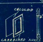
CUT WINDOW OPENINGS IN SIPES & CEMENT CELULOIDE SASH IN PLACE
