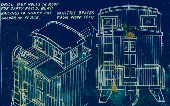
BRAKE HOSE BENT FROM !" DIA WIRE & SOLDERED TO UNDERFRAME. FLATTEN END WITH HAMMER.
