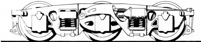
BUCKEYE TENDER w/plain journals, sprung and equalized. 10'-3" wheelbase, 36" wheels U-73 pr.
