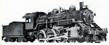
Locomotive data: Overall length including tender, coupler to coupler 18¼". Wheel Base 6½"; Driver diameter 70"; Draw bar pull 17.6 oz; Average speed with maximum load (12 volts) 61 scale, mph; Powered with a 5/8" stack motor; Available in either AC or DC; Minimum radius 32".
