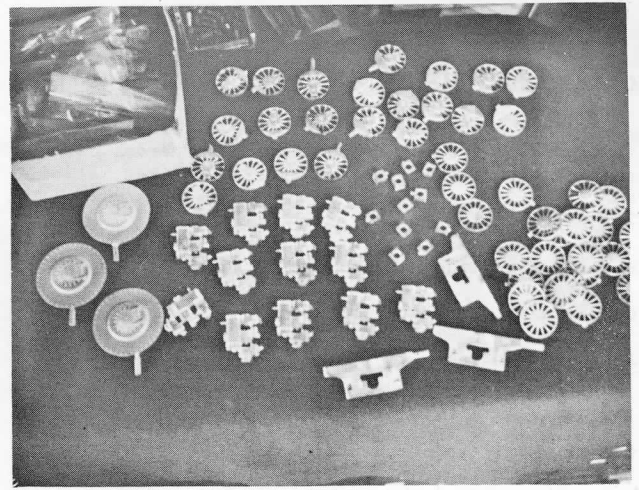
A shipment of lost wax parts - three styles of 63" drivers, BL-2 feed heaters, smoke box fronts, Pennsy pilots & driver journals.
