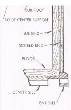
Glue the sub ends to the floor, be sure the rabbet in the floor is up as shown. Glue the sub roof on top of the sub ends. Glue the roof center support to the sub roof; make sure that it is centered on the sub roof.
