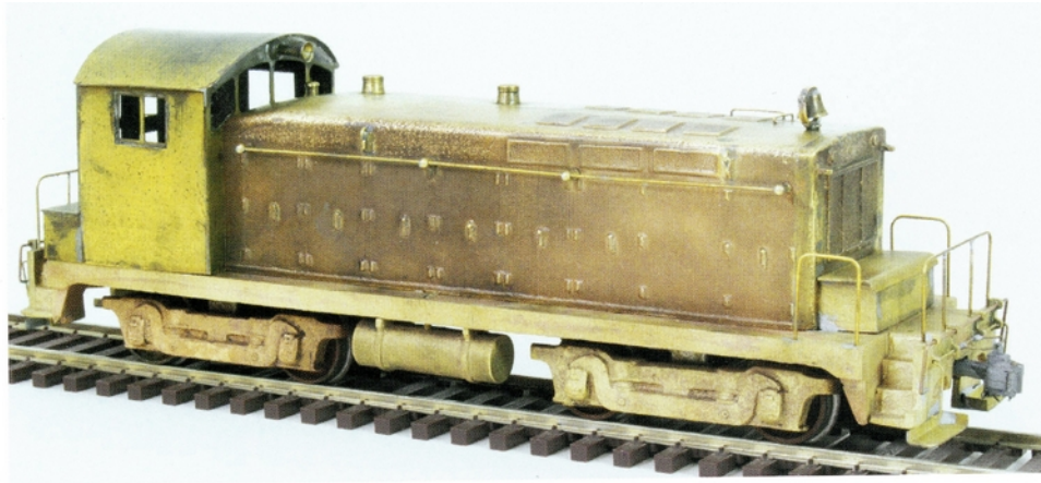
• FIGURE 4: The Hawk EMC SW/SC is a composite model — the hood, frame, and truck sideframes are cast bronze while the cab and toolboxes are formed and soldered sheet brass. No other model is known that is built in this way. The model plans show that headlights, missing here, were provided with the kit.
