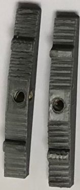
Bolsters, Brass Nuts Embedded (2)
